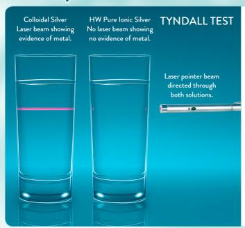
Normally when a laser is shone through a liquid other than distilled water, a path of light can be seen similar to when you shine a torch through smoke or fog.
